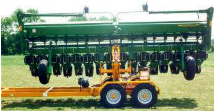
Self-loading implement trailer with a drill being loaded. Photo courtesy of Tensas Machine & Manufacturing.
